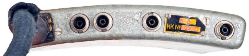
Bottom view of the Neva transmitter-receiver unit showing sockets for battery (B), speaker (T), vibrator (B), and microphone (M). Note the slightly curved shape for carrying the set on the chest.
