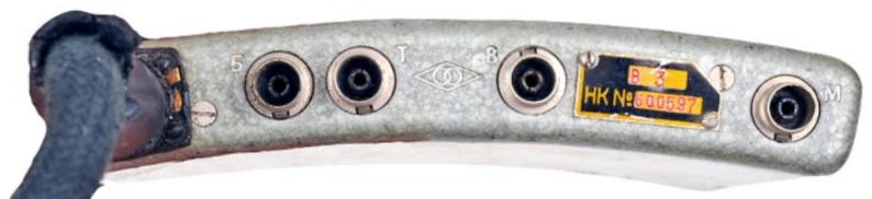
Bottom view of the Neva transmitter-receiver unit showing sockets for battery (B), speaker (T), vibrator (B), and microphone (M). Note the slightly curved shape for carrying the set on the chest.
